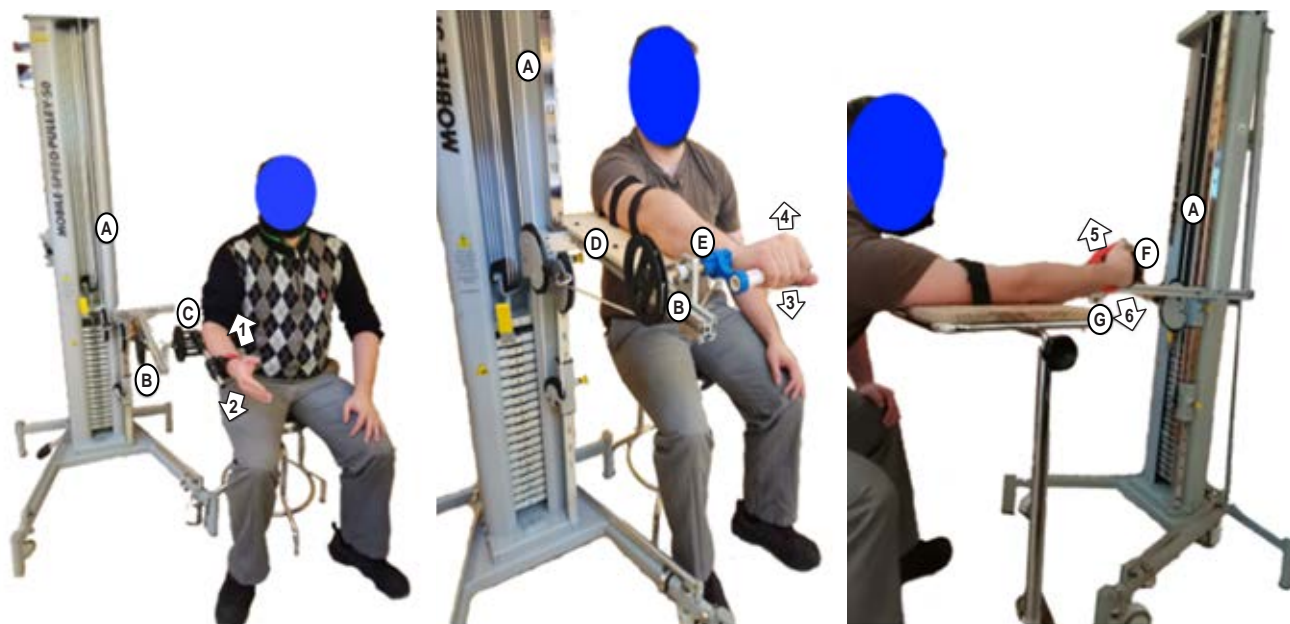
Figure 1: Single-degrees of freedom upper limb movements proposed measurement setups. A) Pulley machine. B) Pulley machine deflection pulley. C) Elbow flexion/extension deflection pulley. D) Arm fixation table for wrist flexion/extension measurement setup. E) Wrist flexion/extension deflection pulley. F) Wrist medial/lateral deflection pulley. G) Arm fixation wrist medial/lateral deviation table. The numbers indicate the movements made. Where 1,2 is the flexion/extension of the elbow. 3,4 is flexion/extension of the wrist. 5,6 is medial/lateral deviation of the wrist.
